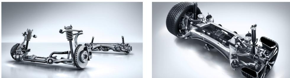
This suspension with selective passive damping system ensures balanced ride comfort by optimising ride characteristics, damping effect and stabilisation according to the road surface conditions.
